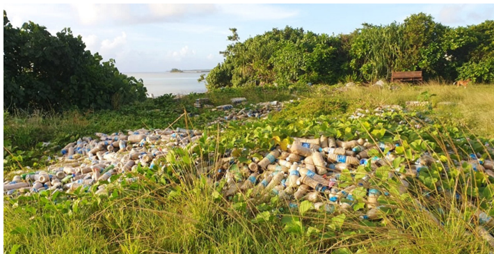
Figure 7: Bottles filled with sand to be used in seawall construction
